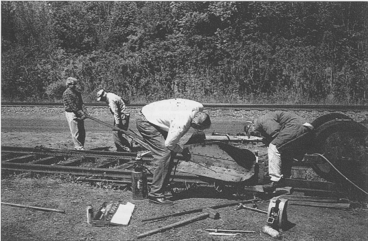
Hank Kaminski and Jim Tomczyk are hard at work removing the plow blade from one of our trucks while, Bob Hooper and Allan Nelson are in the background working on other things. Photo by Tony Hall
