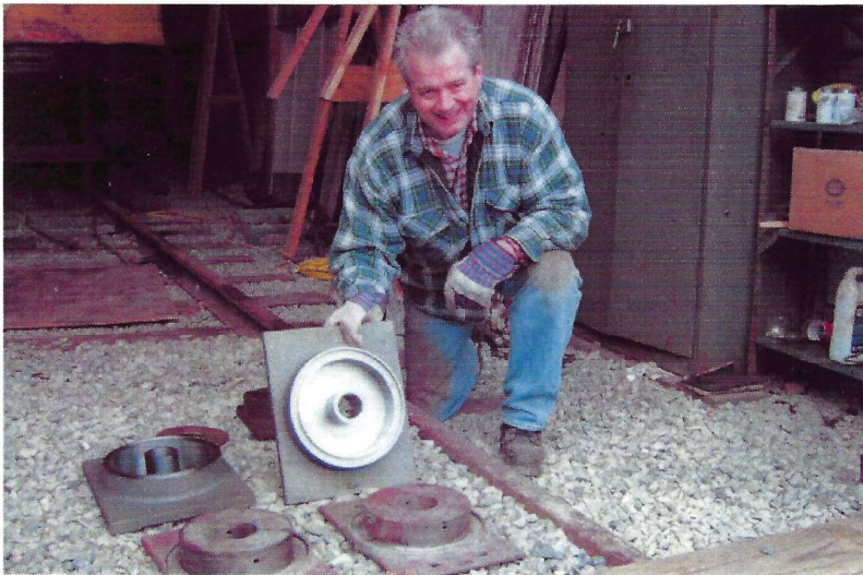
Bob Hooper proudly displays the new center bearings produced by Jim Roberson of L&M Fabrication and Machine of Bath, PA to fit existing counterparts on the bolster beams of 2651. The donation of the center bearing fabrication was a significant contribution to the restoration of the car.
