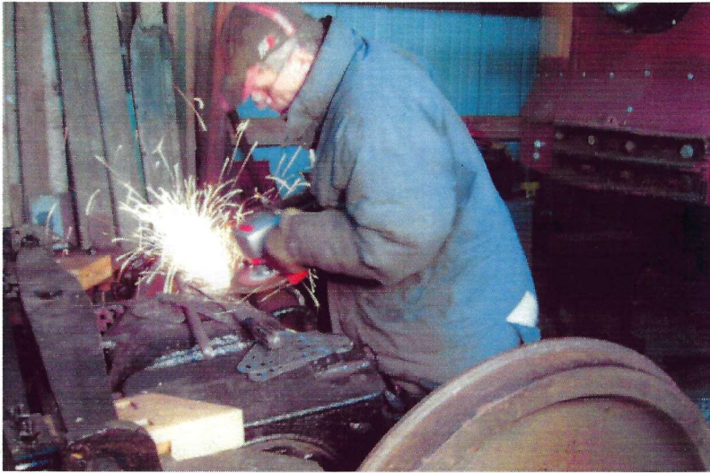
Jim “Sparkle Plenty” Tomczyk grinds new air vent guards he produced in his home shop.
