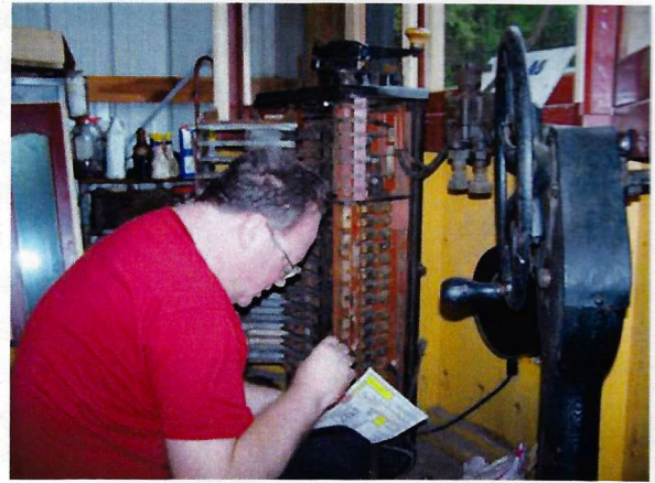
Carl Hosler makes final adjustments to the east controller which in a few moments will spring the car to life for the first time. Tony Hall photo, October 2011.
