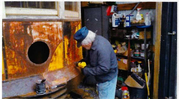
Using the group's newly acquired heat gun, Tony Hall is removing the very paint he helped apply 38 years ago. Bob Hooper photo, 28 January 2012.
