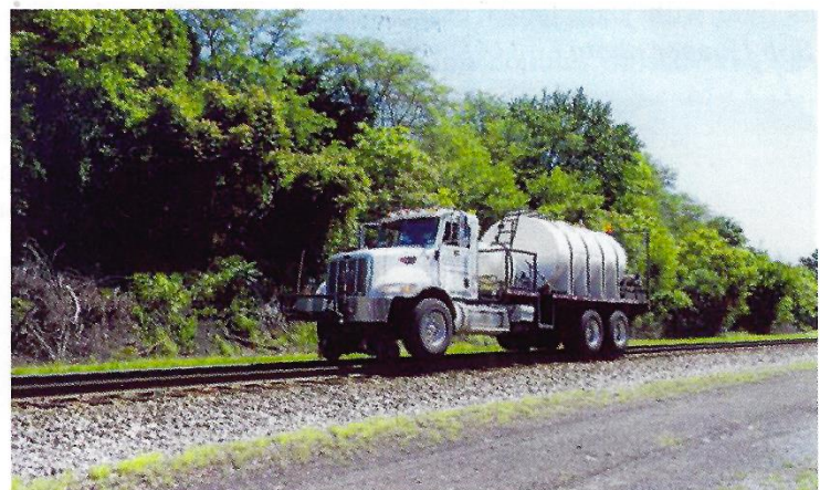
NS weed killer rail truck effectively eradicates unwanted weed growth from its busy ROW. Where's the Toxic Avenger when you really need him? Photo Tony Hall, 18 Jun 2012.
