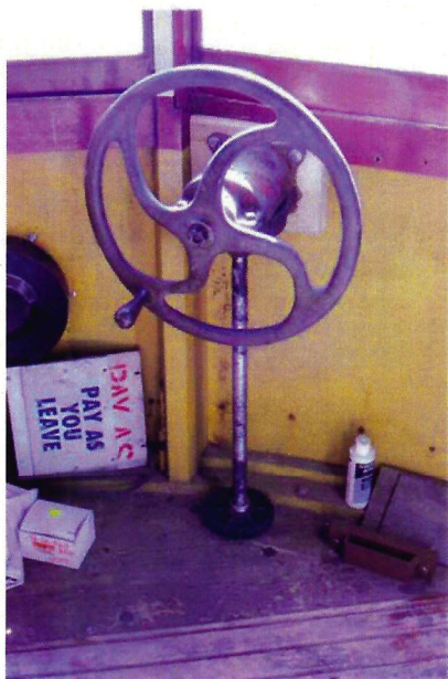
Top: Jim explores National Pneumatic door motors, probably made at their Rahway plant. Mid-left: He goes on to drill a major brake bracket, which he displays, ready to install, at mid-right. Bottom left: After much custom machining, Bob Hooper has assembled the hand brake stands. Bottom right: Work crew pigs out at Joe's Steak House. From left, Bob Hooper, Bill Toikka, Hank Kaminski and Tony Hall. All photos (except lower right) by Tony Hall, January and April, 2013.
