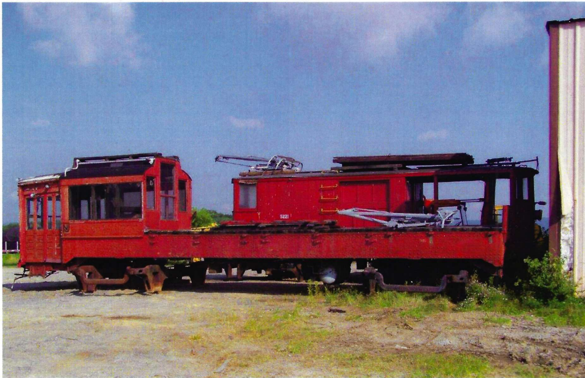
Above: In this recent view taken at Lyons Industries, Ebensburg, PA, both car bodies rest on diesel locomotive truck frames while the motors and trucks are removed to the shop for reconditioning. Photo 19 July 2013.
