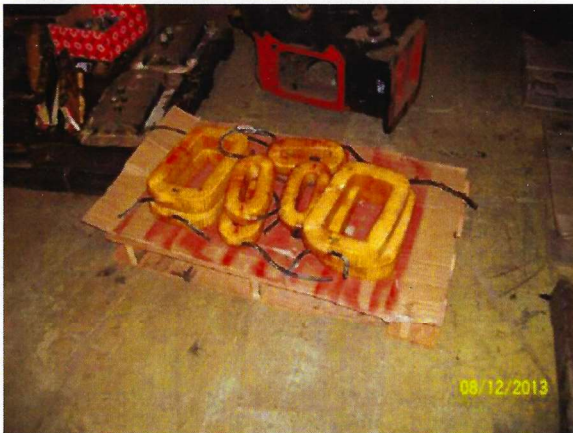
Top left: Motor housings were opened for the first time in possibly fifty years. Top right: Motor cases from 5221 have been disassembled in the Electrical Shop for inspection and repair. Mid left: Motor housings have been cleaned and inspected. Mid right: The motor armatures have been uncased. Lower left: Motor coils from 5221 awaiting inspection. Lower right: Same coils look almost brand new after cleaning.
