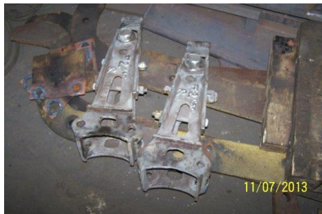
In the above four views, we see (upper left) a main truck frame stripped and made ready for priming and painting. In the upper right view, the unsprung truck frame is being similarly prepared. In the lower left, we see a pair of brake shoe holders stripped to bare metal. Santa was good to us this year, as in the lower right we see a generous supply of new bolts, nuts and small parts left by Old Saint Nick under our Lyons Christmas tree. 7 November 2013.
