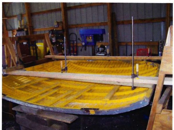
UL: Temporary retaining planks are clamped to the bonnet so that it will maintain its proper curvature during its replacement atop the east end platform. UR: Pressure is exerted across the back of the bonnet so that the curvature will remain correct. ML: Jim Tomczyk makes final adjustments to one of the stiffening bars he will fit into the bonnet base. MR: Hank makes fine cuts to the recession into which the stiffening plate will be fitted. LL, LR: All stiffening bars having been fitted to the bonnet base, the temporary retaining planks are finally clamped into position, assuring the curvature of the bonnet will remain constant and correct during the reinstallation to come. All photos by Bob Hooper, April 2014.
