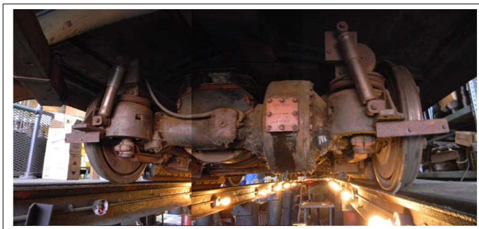
This composite view of #25's undercarriage shows the automotive influence on the PCC design: i.e. the hydraulic shock absorbers and hypoid gears.
