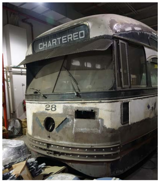
The classic smile of the PCC is diminished by layers of dust and grime at the open HBLRT facility. The front anti-climber has been replaced and body patching begun.
