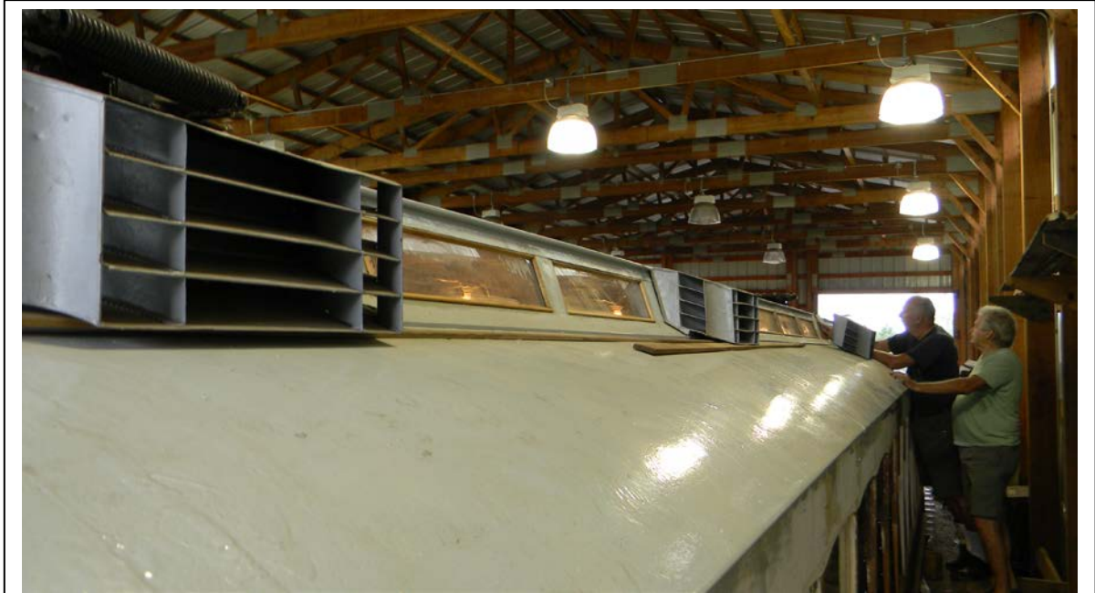
The roof of PSR 2651 shows improvement with the ventilators and clearstory windows installed. In the background, Bob and Hank continue to fit the remaining ventilators.
