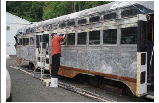
Removing six coats of paint and a lot of Bondo takes a lot of manpower as Bruce Russell demonstrates.
