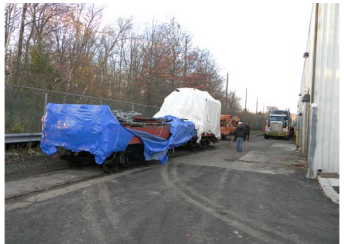
Figure 16: KS Fork Lift pulls Flat Car 5223 to the west end of the storage track to clear the unloading site for 5221.
