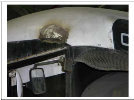
PCC #28's car body required welding repairs at the joints of the window posts, letterboard and roof.
