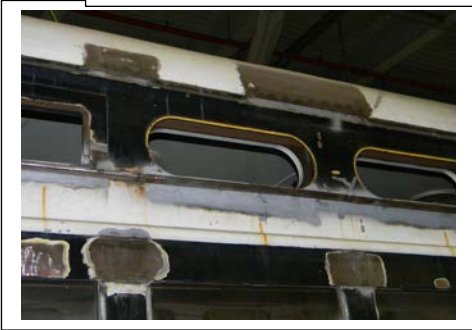
PCC #28's car body required welding repairs at the joints of the window posts, letterboard and roof.
