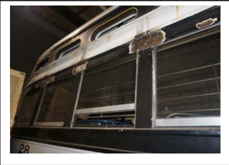
PCC #28's car body required welding repairs at the joints of the window posts, letterboard and roof.
