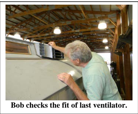
The roof of PSR 2651 shows improvement with the ventilators and clearstory windows installed. In the background, Bob and Hank continue to fit the remaining ventilators.
