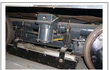
Reconditioned actuators and spring hangers are evident.
