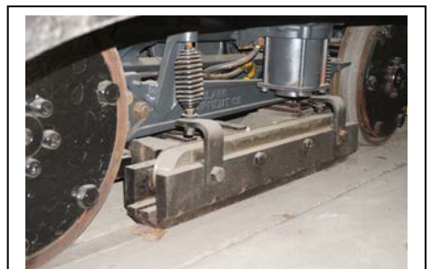
The rebuilt trucks are complete down to the magnetic track brake.
