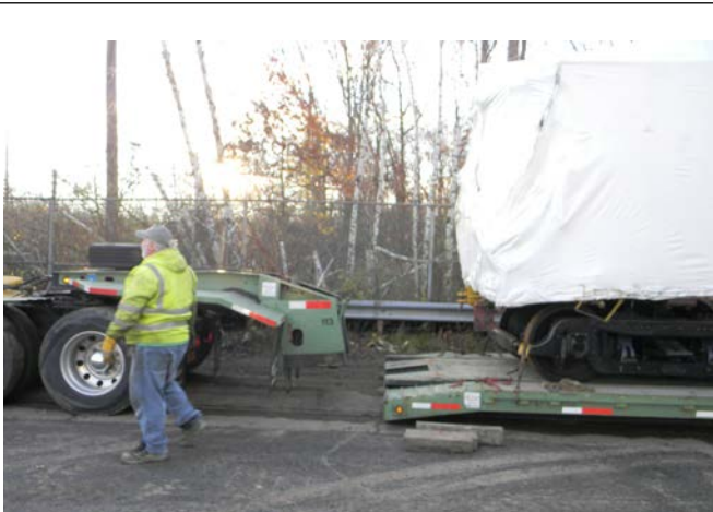
Figure 17: Silk Road Ro/Ro trailer drops its leading edge for unloading
