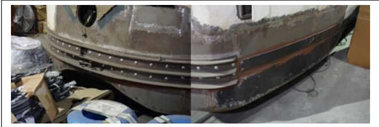
The classic smile of the PCC is diminished by layers of dust and grime at the open HBLRT facility. The front anti-climber has been replaced and body patching begun.
