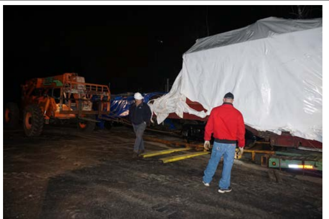
Figure 12: Gingerly, the flat car is inched off the trailer, seen here traversing the unloading ramp.
