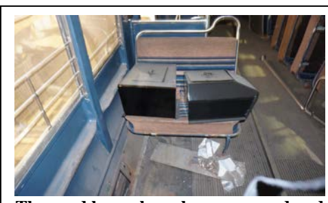
The sand boxes have been removed and reconditioned. A seat assembly provides a temporary storage platform.
