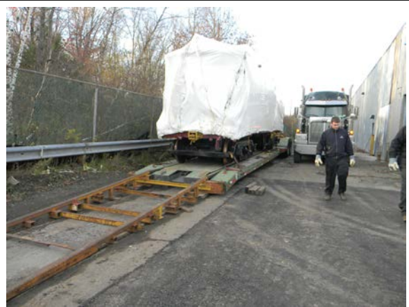
Figure 20: Here she comes, inching down the unloading ramp. A cable played out from the rear mounted trailer winch, restraining the car from running away.
