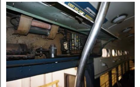
The electric rear door opening mechanism is shoe-horned into the transom above the door opening.
