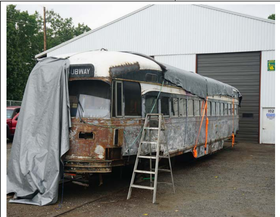
With the majority of the paint removed, the body patching can begin as you can see by the welded plate on the roof over the operator side window. The lower corner panels are next to be attacked.
