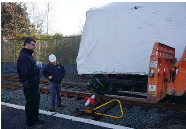
Figure 23: The first truck of line car 5221 passes a track switch as the second truck "touches down".
