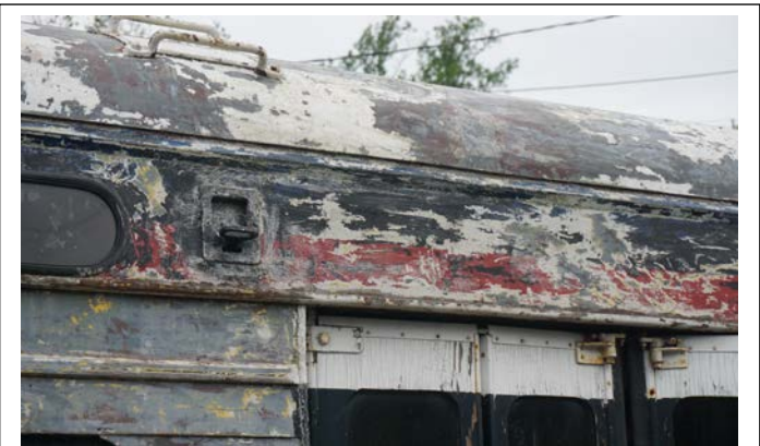
The car body still carried six paint schemes applied previously including the TCRT Yellow, visible if you looked closely.
