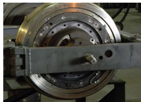
As KS follows their maintenance manuals to the letter, you have specialized equipment for every job. Here we see a wheel puller jig for a stub axle. These are re-greased every 155 km.
