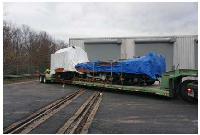
Figure 8: In reverse, it was possible to negotiate the tight turn at the end of the building where the unloading track was located, seen in the far left.
