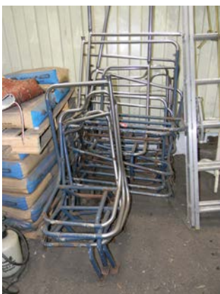
Seat frames seem to glisten seductively, but in reality will require repair of significant rust damage.
