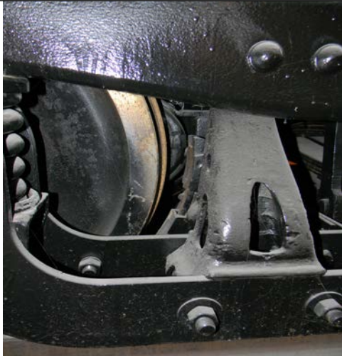
#5221, upon arrival from Lyons Industries, was found to be short a brake shoe.
