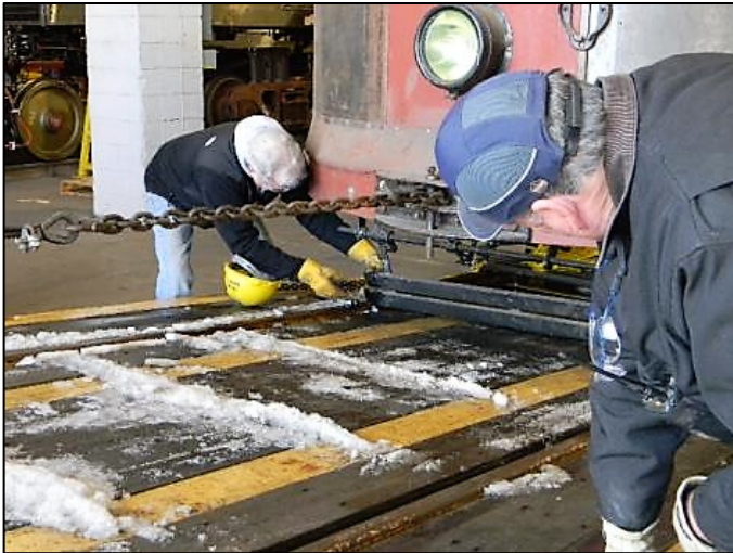
Fig. 15-3. Again, safety appliances must be adjusted to clear the steep loading ramp. That’s real ice in the gauge.
