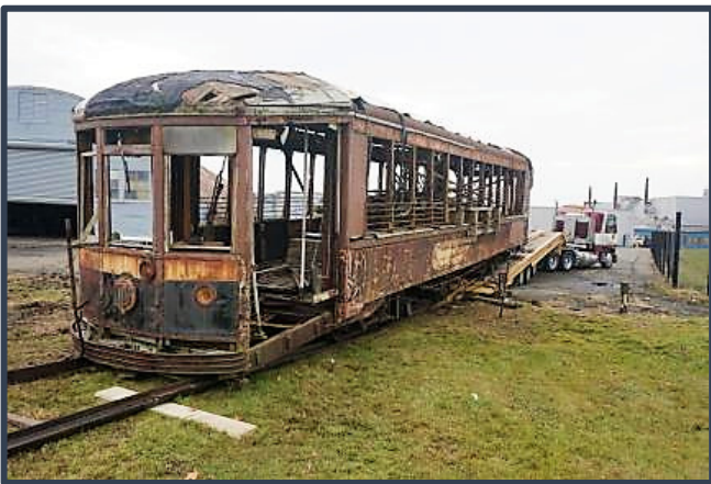
Fig. 19-3,4. Sagging end platforms fouled on the storage rails.
