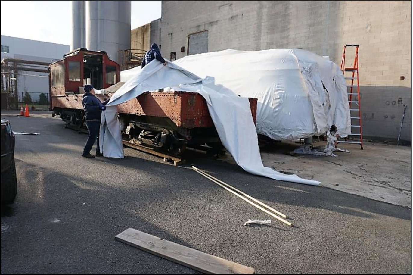
Fig. 13-1. With our three cars on the outside panel tracks, the shrink wrapping can begin.
