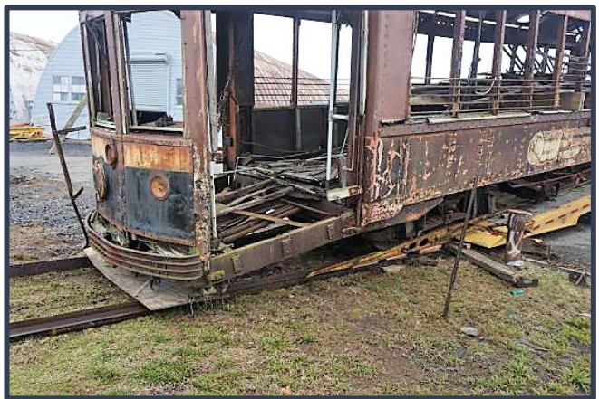
Fig. 19-3,4. Sagging end platforms fouled on the storage rails.
