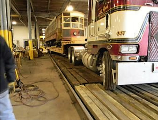
Fig. 18-1. The trailer, with load, had to be SKIDDED SIDE-WAYS with K-S’s huge forklift.
