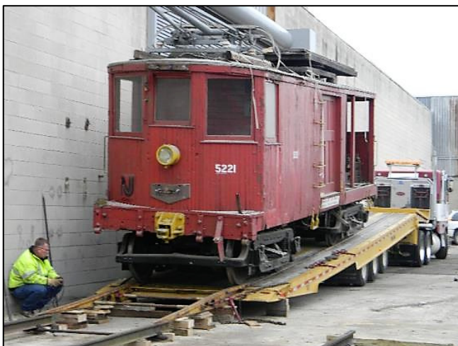
Fig. 11-5. Slowly, ever so slowly, #5221 is unloaded without incident. Practice makes (almost) perfect.
