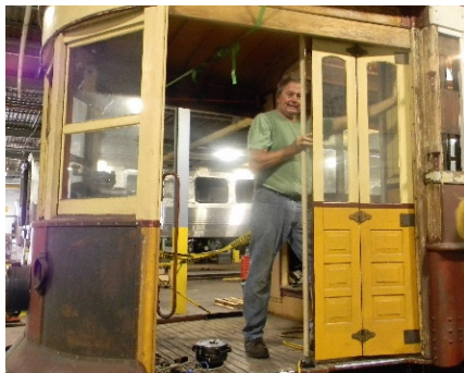
Fig. 20-5. Bob Hooper test fits the first of four doors.
