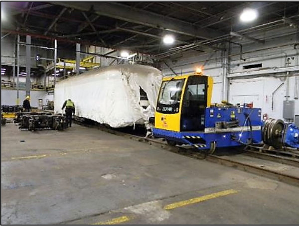
Fig. 12-1. PCC #1, still in the Arkport Shrink-wrap, is moved across the plant floor to the exit door with the help of KS's Trackmobile.
