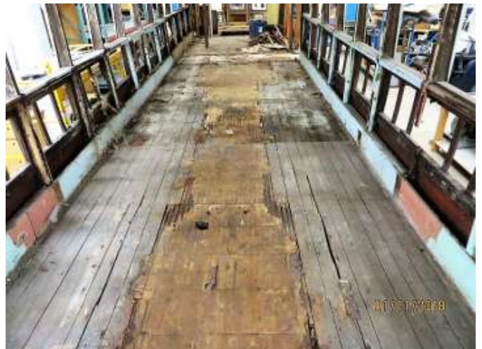
Fig. 12.4 The interior seating arrangement was changed during its service life, and those changes were visible in the holes left over from seat pedestals long since removed. (Keigher Collection pt3-2)
