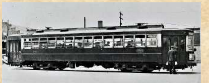
Fig. 6.6 Car 364 is at the SW&A carhouse for a crew change. Note that the side route sign box has been surgically removed, a modification not done to all Windsor cars. (Edward T. Francis Collection P151-dr)
