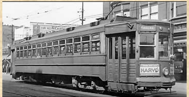
Fig. 8.6 Windsor streetcar, number once again obscured, is buttoned up for a cooler season and shows her surgically-removed route sign boxes. Air whistles and dual markers were added to the upper dashes above the doors. (V3)
