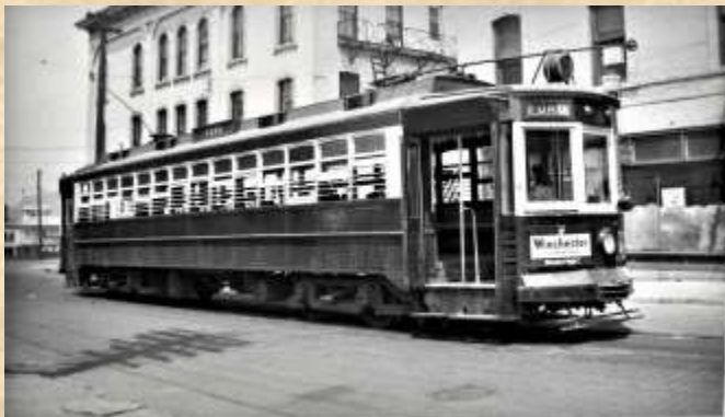
Fig. 8.3 With number obscured, this summer shot shows an EFC car sporting an interurban headlight, typical of cars assigned to the busy "FORD" line which served the automaker's vast Windsor works. (Keigher Collection p152-r)
