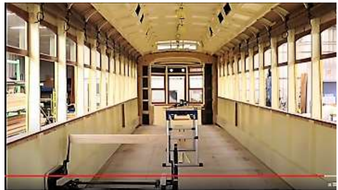
Fig. 14.4 Car 351 interior during restoration, revealing the seating pattern characteristic of the cars during Windsor service. (V12)
