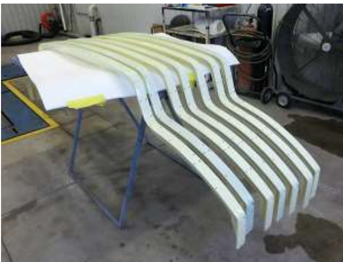
Fig. 12.5 Seven of the original steel roof formers have been cleaned up and painted. (Keigher Collection pt4-2)
