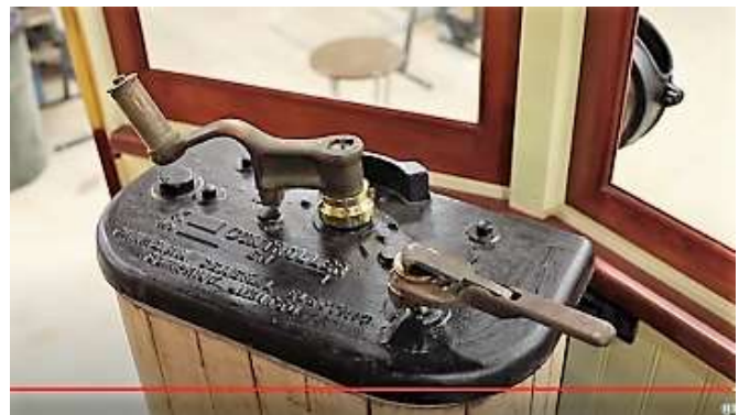
Fig. 14.6 Car 351 K-35 controller head. At center: throttle handles. At right: the Off/On Forward & Reverse switch. Note the mounting of the trolley-catcher, outside the window, within reach of the crew inside the car. This feature was welcomed by operators who were required to change ends during a frigid Canadian winter, when venturing outside might have required snowshoes. (V14)
