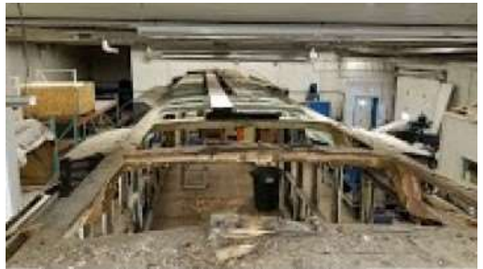
Fig. 12.2 The steel roof ribs were sheathed with a Homosote predecessor called "Agasote." (Keigher Collection Pt3-3)
