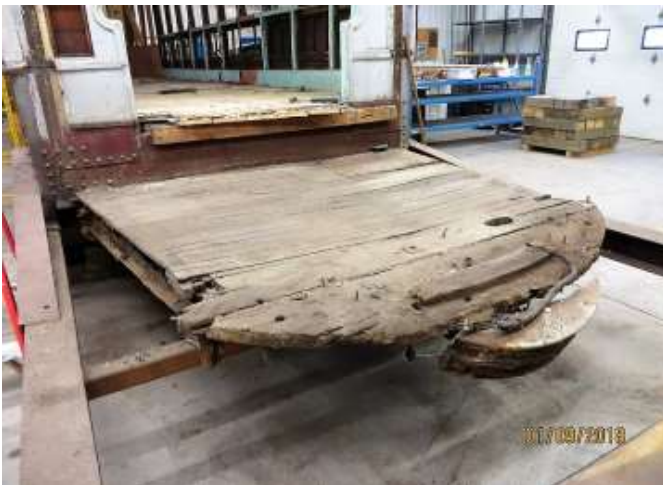
Fig. 12.3 Not much is left of the car's platform, but there is evidence of long-gone controllers and brake stands. (Keigher Collection pt3-1)
