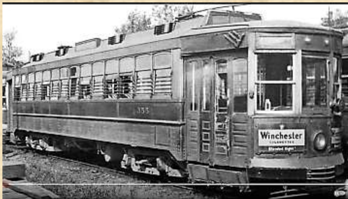
Fig. 8.5 Windsor Car 355. Roof sign boxes are still intact. Minor refits made to EFC cars were not entirely consistent. (V5)
