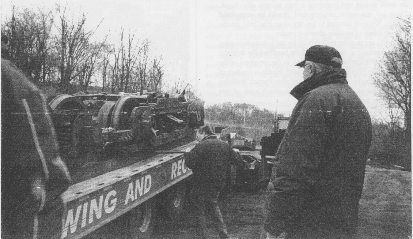
Hank Kaminski stands in the foreground watching the delicate maneuver of unloading one of the trucks from tilt bed trailer ramp and the track in front of the building housing the 2651. Bill Wall stands next to the trailer ready to coax the truck along.
